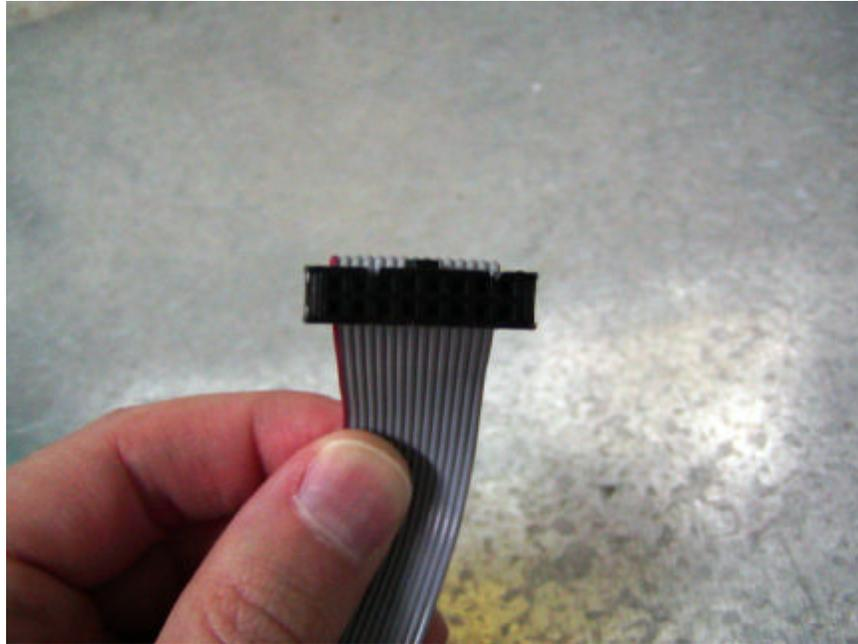
The JTAG connector end (old cable from a PC card)
